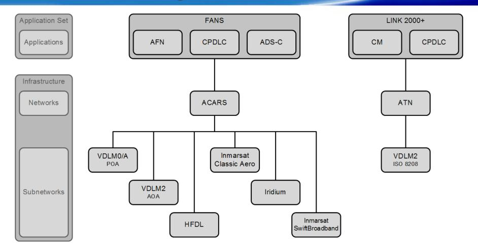
FANS applications are independent from ACARS router, which switches between subnetworks to maximize communications availability according to operator preferences
